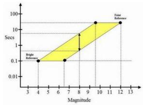
From these observations, we can establish a range of acceptable guiding exposures. The parallelogram seen in the figure to the left represents this region as bounded by the two reference points. If we consider an 8th magnitude star, the exposure could range
