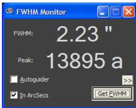
Note that the Peak Value display in FWHM Monitor is not exactly the same as the image maximum value: the peak value is the maximum value of the selected star, not the whole image.
